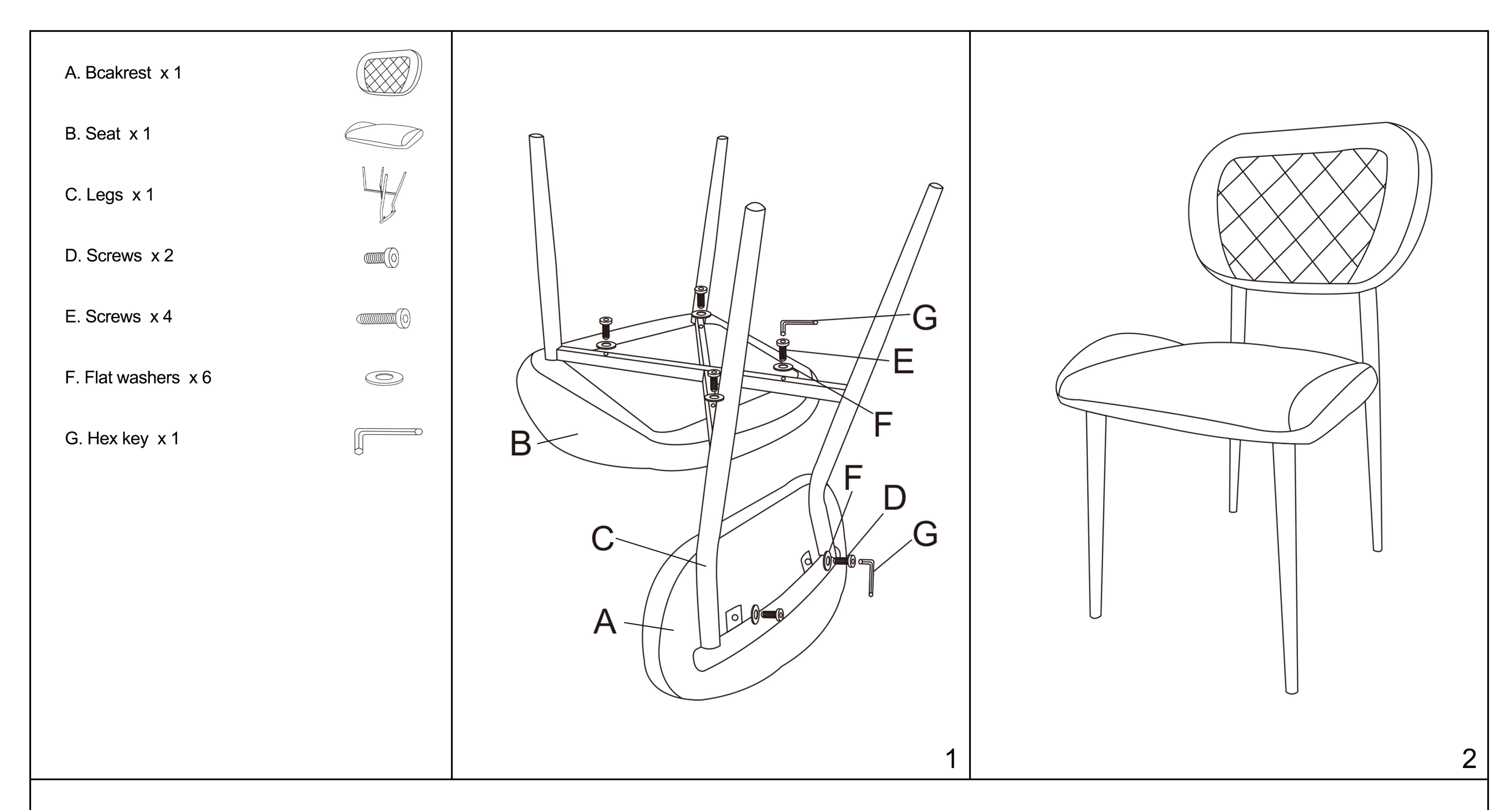
Remark: First fix screws lightly by hand and at the end of the assembly fasten the screws firmly with tools.
