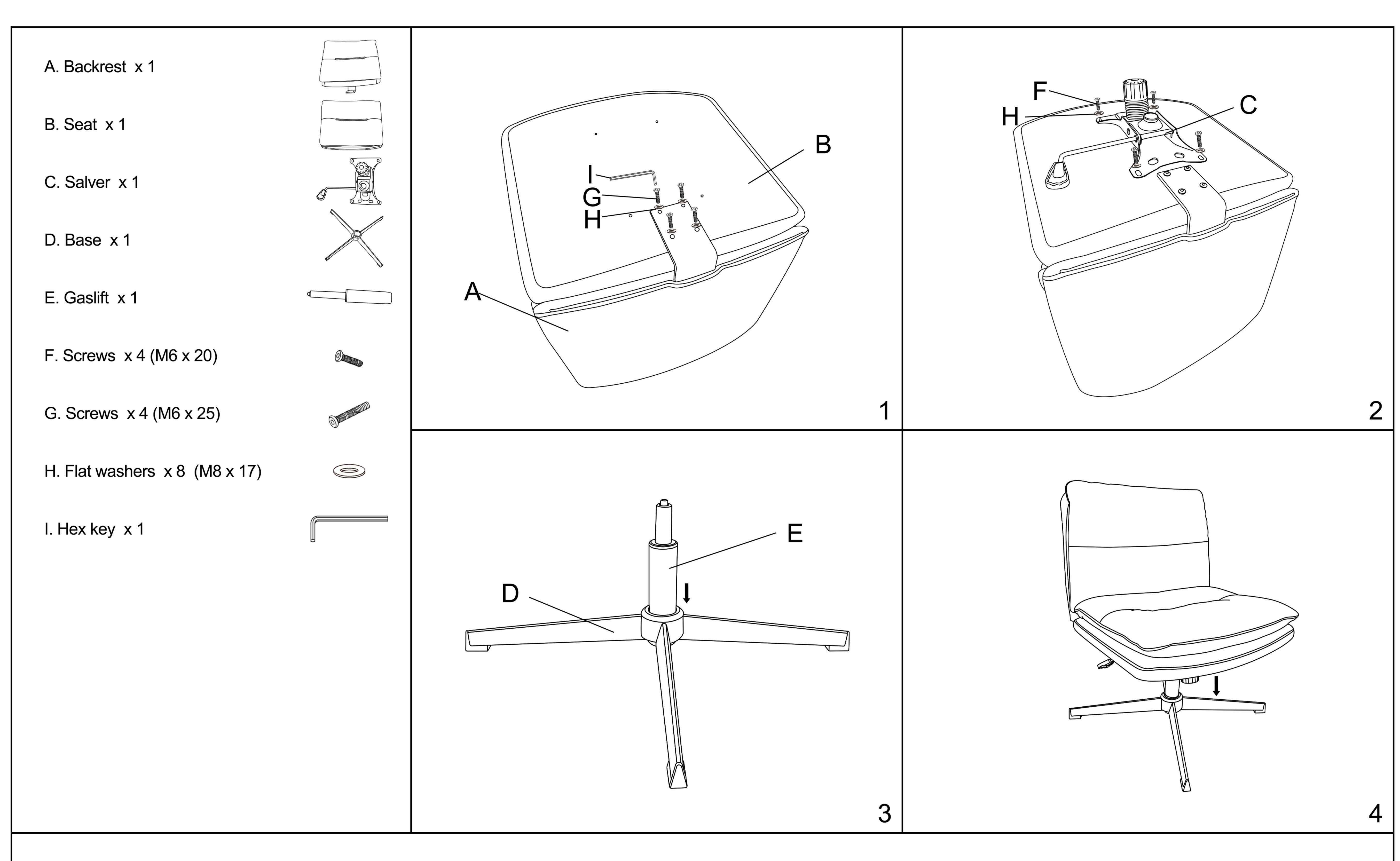
Remark: First fix screws lightly by hand and at the end of the assembly fasten the screws firmly with tools.
